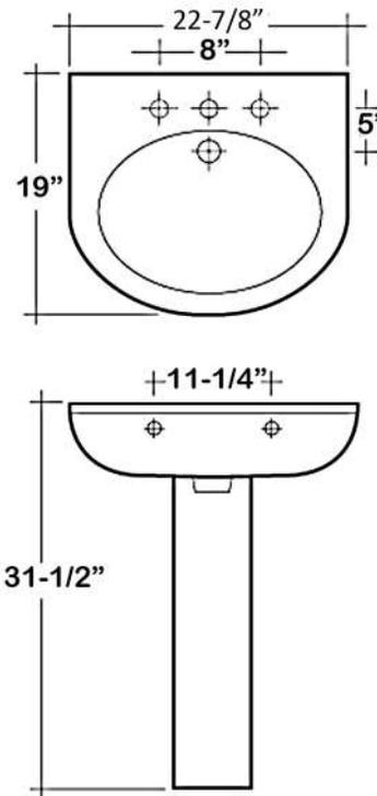
Dimensions of fixture are nominal and may vary within the range of tolerances established by ASME Standard A112.19.2-2018. Dimensions and specifications subject to change without notice.
