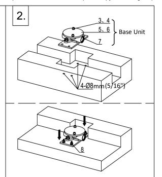
Place the base unit in the mounting hole and mark the 4 drill holes accordingly. Remove the base unit and drill Ø8mm (Ø5/16") holes on the marks. Replace the base unit and insert the expansion plugs (8) through the holes.
