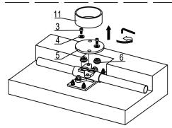
Connect the base to the water supply and flush to check for leaks with water pressure ≤ 1.6 MPa (232 psi). Make sure there's no leak, then assemble the protective ring (11) to the base. Furnish the floor. When cement is dry, remove the protective ring, screws (3), spring gaskets (4), shield (5), and rubber plugs (6).
