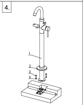
Assemble the shower main body to the base as shown in figure 4.
