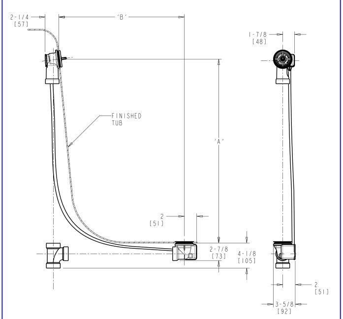
DIMENSIONS ARE IN INCHES AND [MILLIMETERS].
