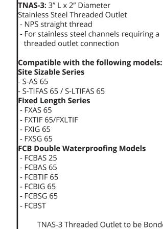
TNAS-3 Threaded Outlet to be Bonded to Stainless Steel Channel using M1 ZSIKA Sealant
