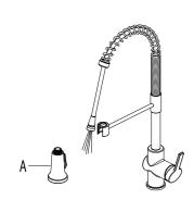
**NOTE**: Please make sure washer is installed attaching spray head to hose.
