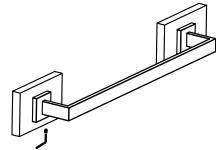
Tighten set screw with allen key (supplied).
