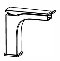
Single-Handle Lavatory Faucet NOTE: THIS FAUCET IS DESIGNED TO BE INSTALLED THRU 1 HOLE,  $\Phi$ 1-3/8" MIN.
