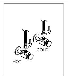
5. Attach flexible hose to water supply.
