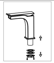
1. Remove the rubber washer,metal washer and locking nut from the faucet.
