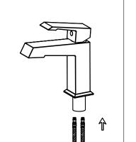
2. Screw and hand tighten the hot and cold flexible hoses to the faucet.DO NOT use a wrench to tighten hoses as this may damage the hose and/or the hose threads.
