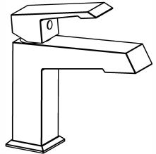
Single-Handle Lavatory Faucet NOTE: THIS FAUCET IS DESIGNED TO BE INSTALLED THRU 1 HOLE, Φ1-3/8" MIN.
