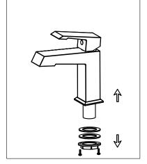
1. Remove the rubber washer, metal washer and locking nut from the faucet.
