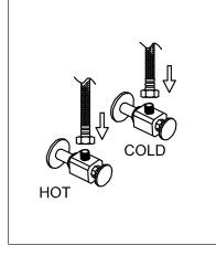
5.Attach flexible hose to water supply.
